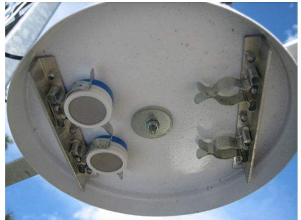
Above. Passive samplers for gaseous pollutants such as \text{NO}_2 and \text{O}_3 are attached to the underside of a rain shield. They are usually exposed for periods ranging from one week to one month and then analysed in the laboratory to determine the average concentration over the exposure period
